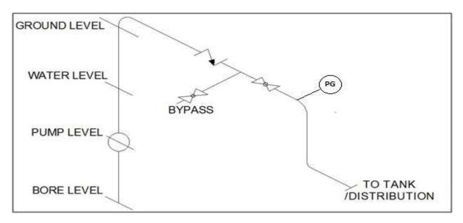
Figure 4: P&ID diagram for New Water Intake plant
