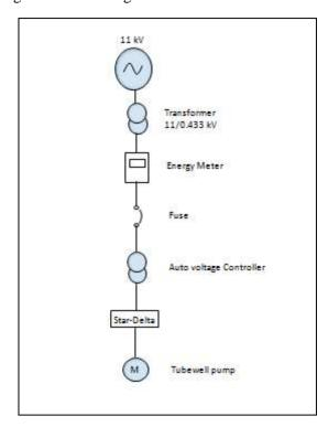
Figure 3: SLD of water pumping station
